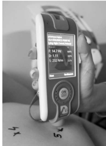
Fig.2. Trapezius muscle during measurement with MyotonPRO device.
