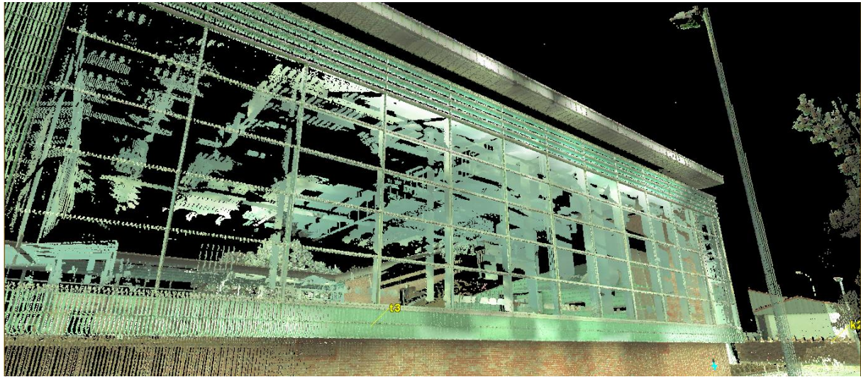
Fig. 2. Deformation of a point cloud caused by the reflection of a laser beam from a glazed wall of the University Swimming Pool in Olsztyn. (source: authors)
